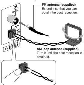
• If the AM loop antenna wire is covered with vinyl, remove the vinyl to expose the tip of the antenna by twisting the vinyl.
